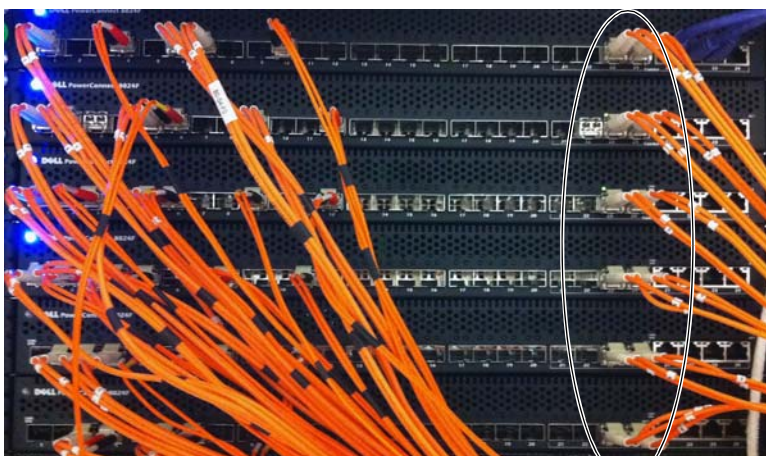
Figure 8-1. Connecting a Stack of PowerConnect 8024/8024F Switches
